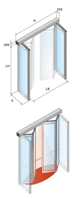
Motion detectors offer a contactless entrance. Further control elements as push-buttons, pull switches or contact carpets can be connected according to the situation. By means of the program switch Bedis you can select the door functions "Manual-Automatic-Open-Night-Exit". Light barriers / scanning safety beam and auto-reverse mechanism make sure one can enter safely.
